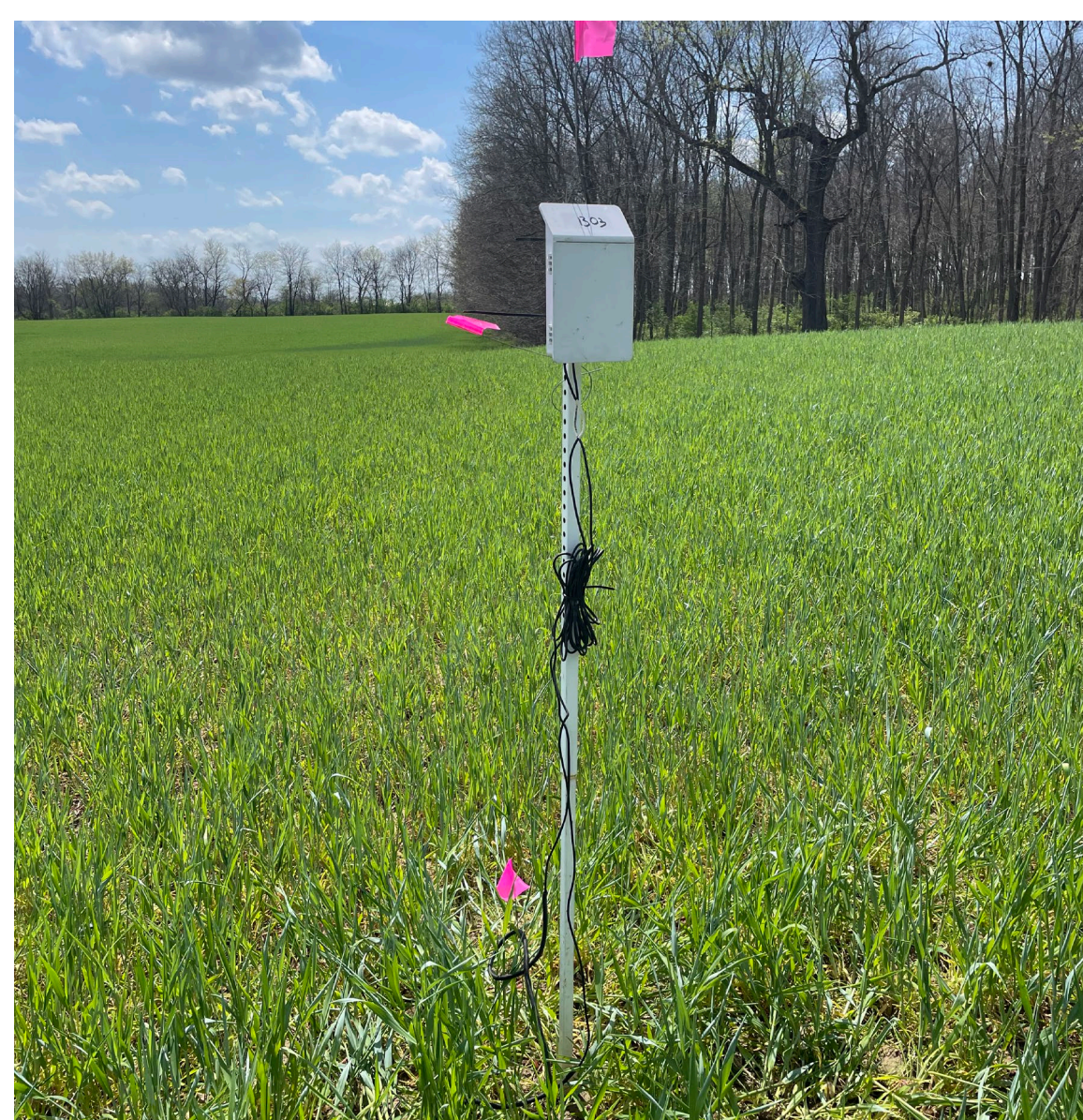
Figure 1. Data logger and sensors installed in cover cropped field prior to termination (left) and sensors placed at soil depths of 2 inches and 4 inches (right).
