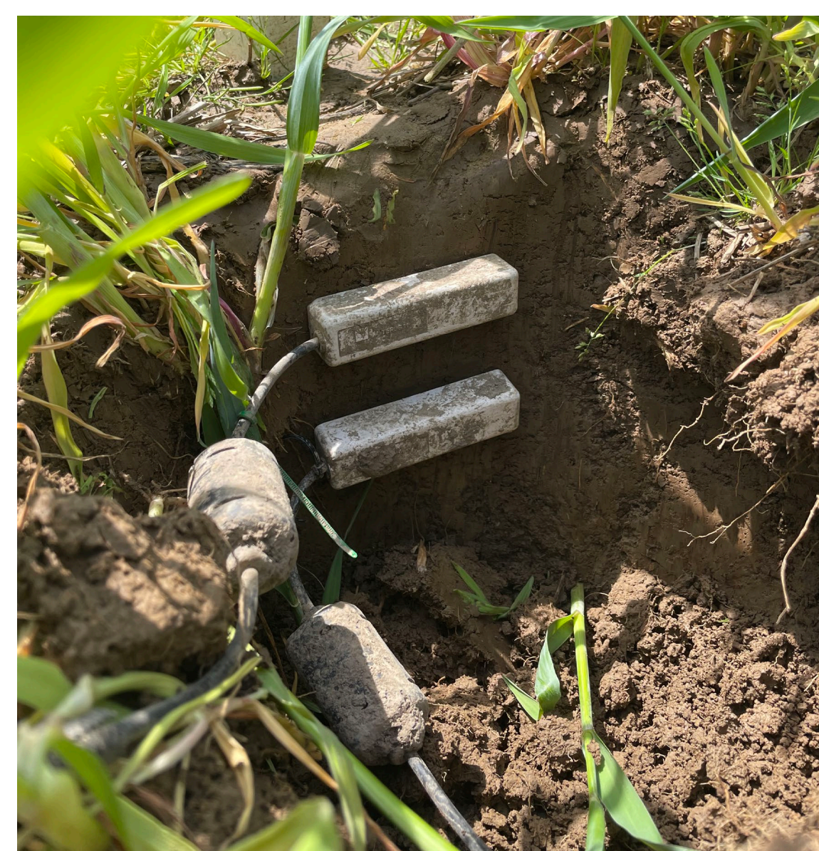
Figure 1. Data logger and sensors installed in cover cropped field prior to termination (left) and sensors placed at soil depths of 2 inches and 4 inches (right).
