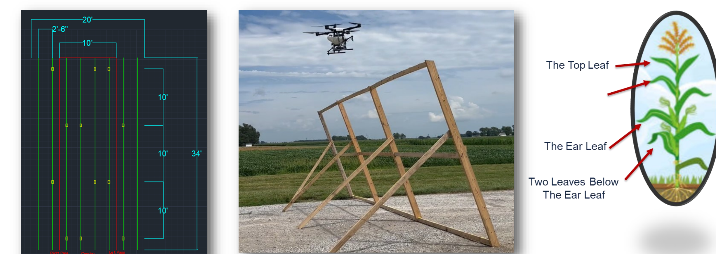
Layout of an on-farm research UAS sprayer project. Spraying water sensitive cards with the UAS for an altitude and swath width study. Water sensitive card placement for in fields fungicide treatments.
