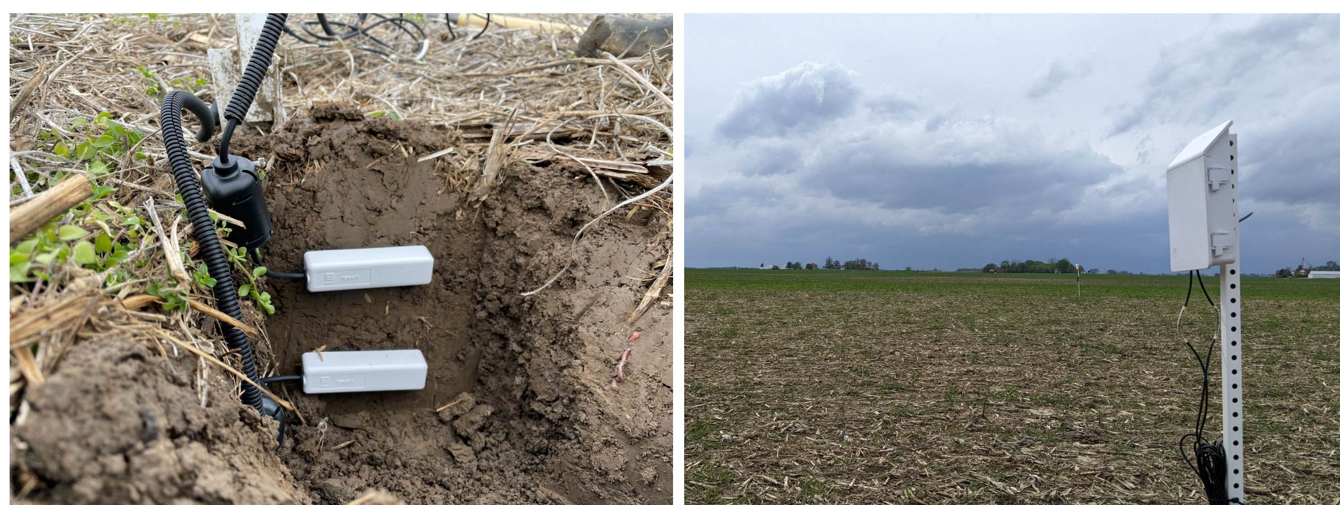
Figure 2. Left- TEROS 11 sensors at 3" and 6" depths. Right- The ZL6 data logger recorded measurements every hour. Cereal rye was the cover crop used in all CC fields at a seeding rate of 20-25 lbs/ac and terminated just before or after planting.
