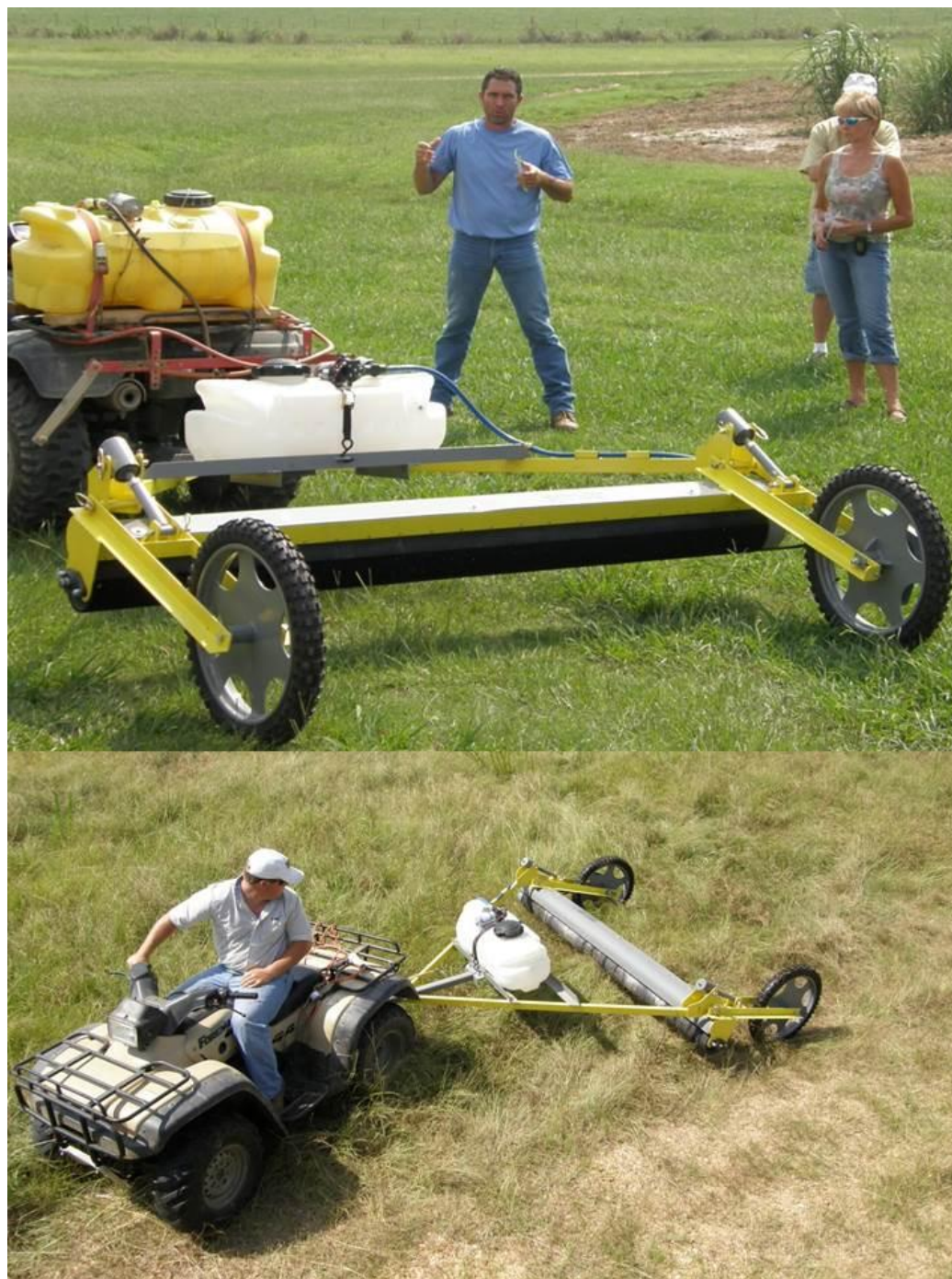
Figure 1. The GrassWorks Weed Wiper (GrassWorks Manufacturing, LLC, Strafford, MO) is an herbicide applicator that can be pulled with an all-terrain vehicle (ATV) or mounted in a tractor. It can be adjusted to different heights to target undesirable weed species without harming desired forage crops. The weed wiper includes a steel rotating drum that is covered with a specialized synthetic carpet-like material and wetted by a 12-volt pump. In the pull-type model used in this study, the rotating drum is powered by a ground-drive system. Any possible chemical drip is minimized because the rotating drum turns at a constant speed in the opposite direction to which the weed wiper is traveling. A shielded boom sprayer is positioned over the rotating drum and it keeps the rotating drum saturated with chemicals and eliminates any potential drift issues. When the operator sets the ATV at the correct speed and drives across the field, the drum passes over the weeds and the touch of the plant releases the herbicide from the absorbent cover. The rotating drum will not physically damage the weeds, but larger plants exert more pressure against the drum and therefore receiving a proportionately larger chemical dose. The advantage of the weed wiper is that it allows the use of selective herbicides for a better weed and bush control in pastures.
