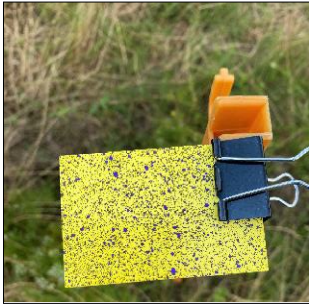
Figures 8-9. Droplet patterns for the aerial and ground applicators in Van Zandt County.
