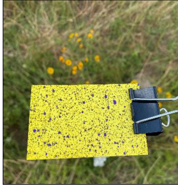
Figures 8-9. Droplet patterns for the aerial and ground applicators in Van Zandt County.
