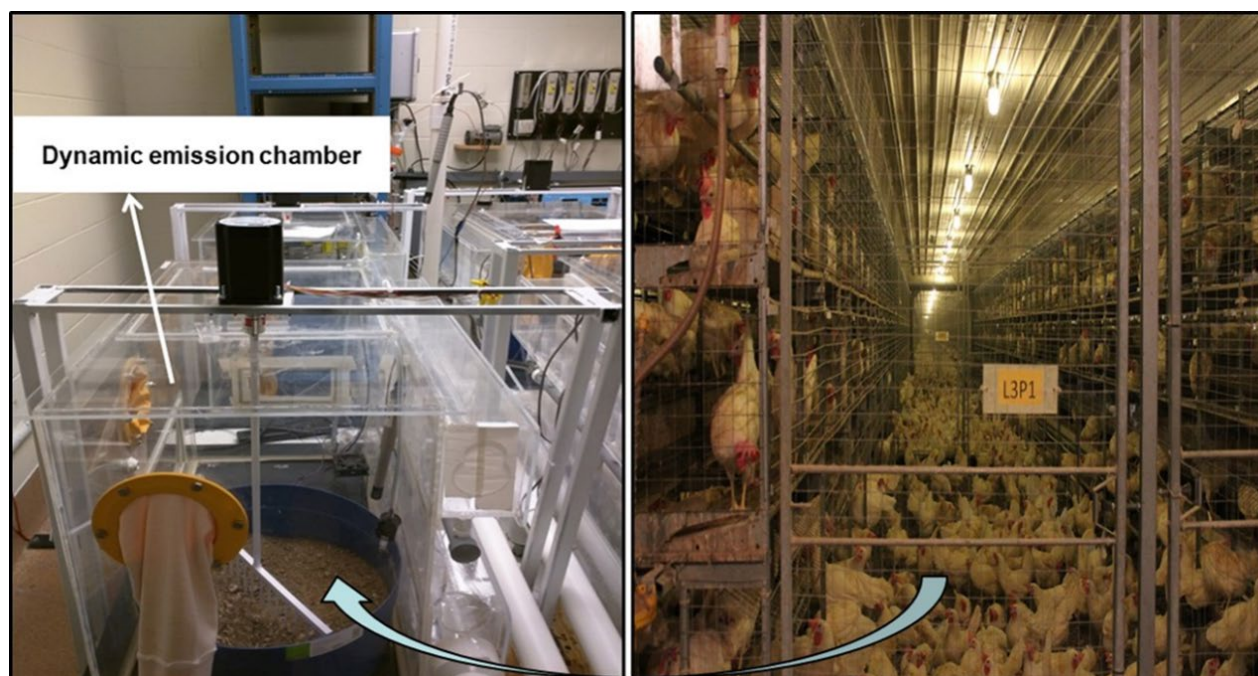
Figure 5. NH 3 mitigation test with dynamic emission chambers.
