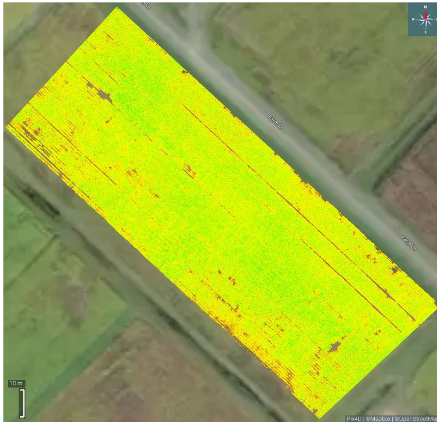
Figure 3. NDVI processed with drone imagery collected using multispectral sensor.
