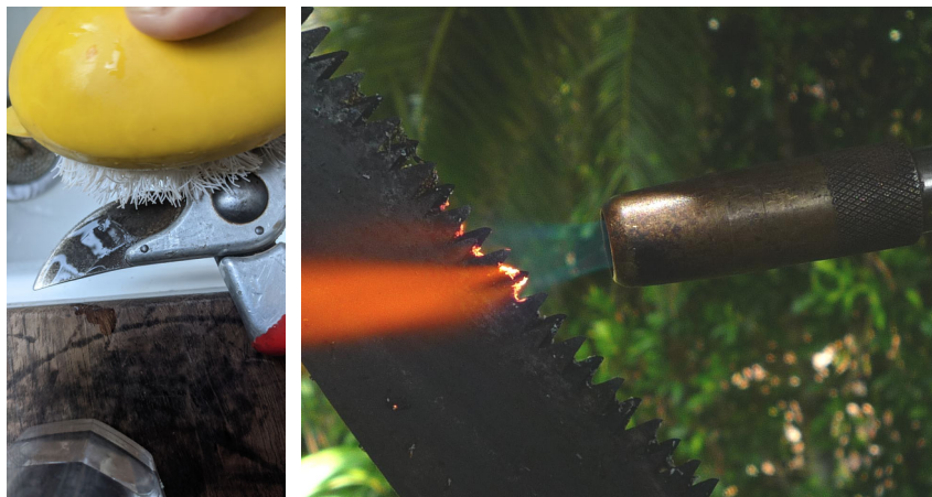
Figures 29-30. A simple scrubbing with a stiff brush (Figure 29) is often all pruning tools need; if there are concerns about transmissible diseases, a quick flaming of the metal blade (Figure 30) will sterilize the surface. Photos by A. J. Downer.
