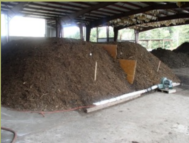
Fig 27. Static composting system. Temperatures must reach 131 °F for 3 days and the piles must be turned 3-5 times.
