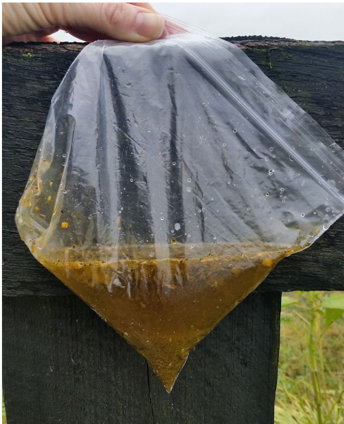
Figure 2. Sand has settled to the bottom of the manure/water mixture. Photo courtesy of proequinegrooms.com
