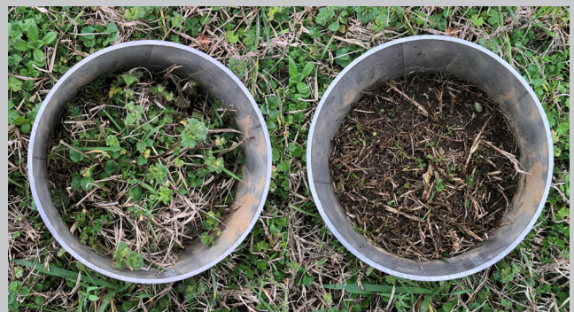
Fig. 3. Removing material from inside the infiltration ring.
