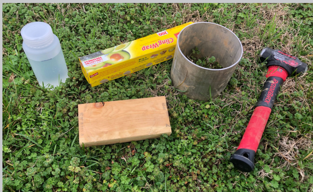
Fig. 1. Materials needed for measuring infiltration rate in the field.
