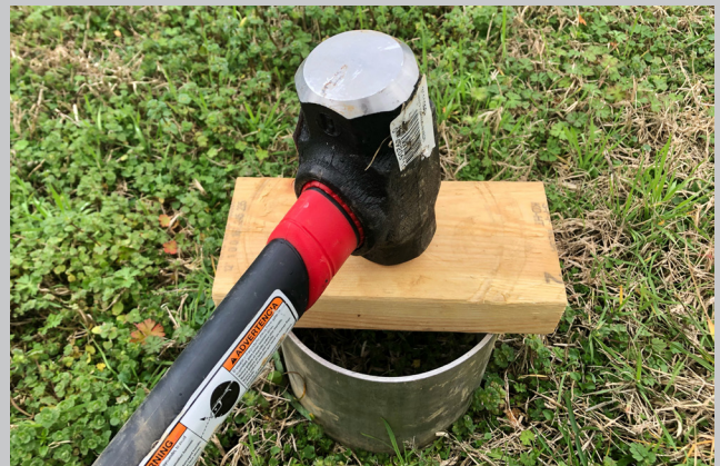
Fig. 2. Installation of the ring using a sledge hammer and wooden block.
