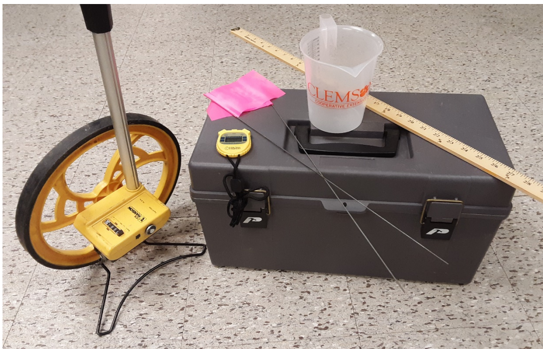
Figure 6. Materials needed for calibration include flags or cones, a stopwatch, measuring cups, a measuring wheel or tape, and a ruler. Photo credit: Justin Ballew, Clemson University (2020).
