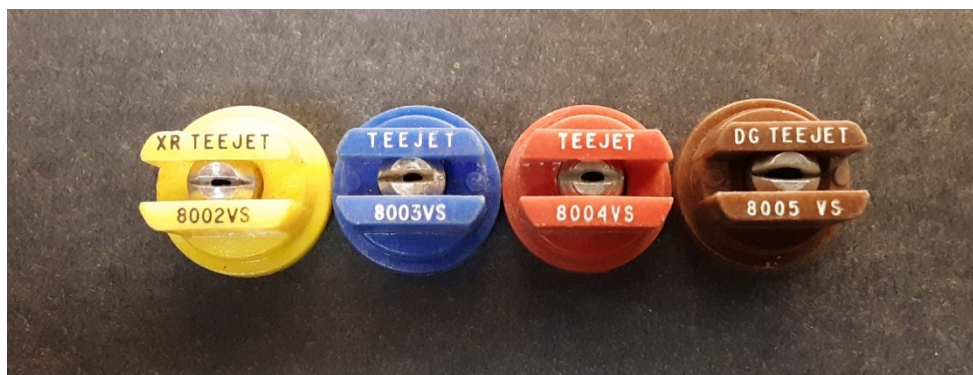
Figure 5. Flat fan nozzles of varying orifice size. The last two digits of the number printed on the nozzle tell the nozzle output. For example, an 8004 nozzle has an output of 0.4 gallons per minute at 40 PSI. Photo credit: Justin Ballew, Clemson University (2020).
