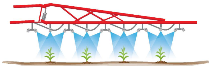
Figure 3. In a directed application with multiple nozzles on a low growing crop, the nozzles are angled to direct the spray into the crop canopy from multiple directions. Image credit: Bek Diamond, Clemson University (2020).
