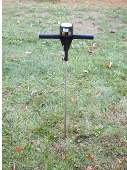
Figure 3: A static cone penetrometer, a.k.a. soil compaction tester. (Photo Credit: Steve Yergeau)
