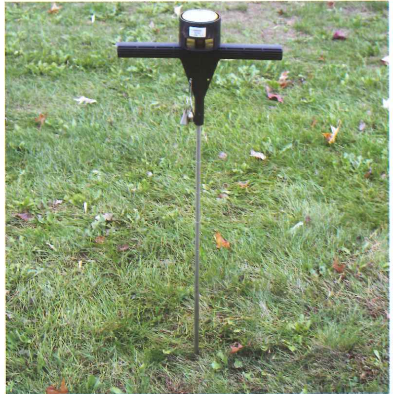
Figure 3: A static cone penetrometer, a.k.a. soil compaction tester. (Photo Credit: Steve Yergeau)
