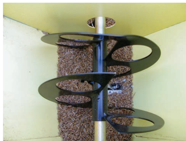
Figure 5. Agitators in the bottom of native grass hopper boxes ensure that the fluffy appendages (awns) on the seed of some native warm-season grasses do not prevent properly metering seed.
