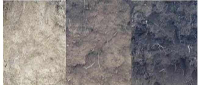
Figure 7. Examples of soil with less than 1%, 2% and 3.5% organic matter. (Jodi DeJong-Hughes, UMN Extension).
